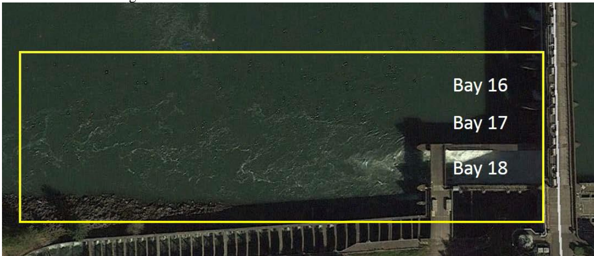
Figure 1. Area of interest for the LIDAR and hydrosurvey of the B-branch erosion issue on the south side of the spillway.
